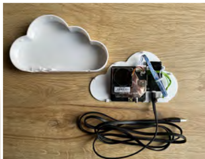
Cloud-shaped window-mounted air quality monitoring station developed by Russian industrial designer Kristina Loginova (used with permission)
