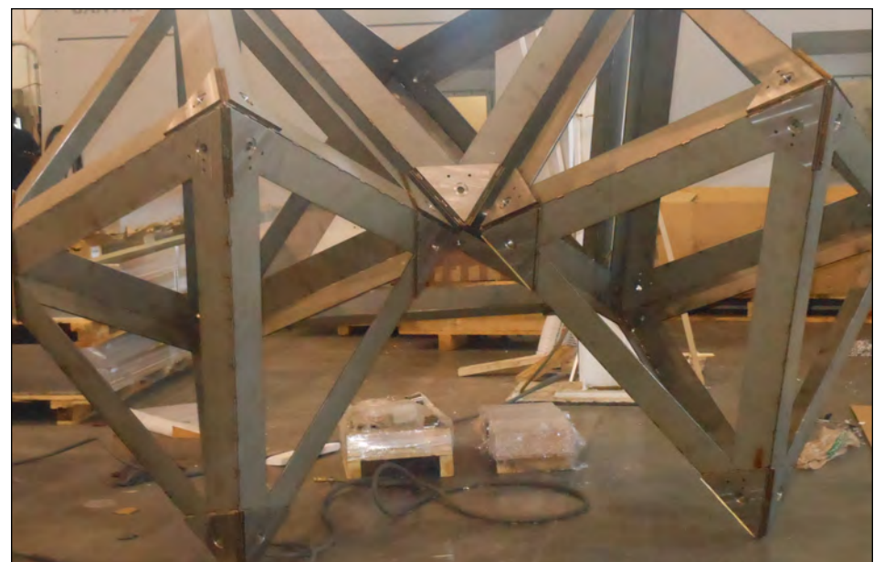
The abstract monument at the A&A Industries' plant, before the triangular plates are installed on the skeleton
